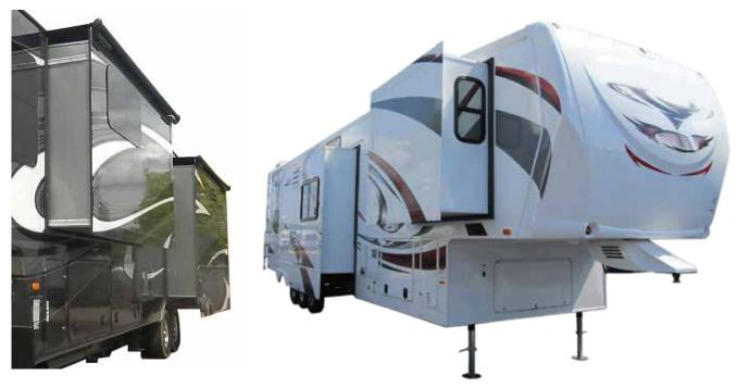
Boyd's patented RV seals solve water, dust and wind ingress problems for slideout room environmental seals, bottom pans and wipers and accessories like serviceable D seals, corner moldings, screw covers and floor transitions.
